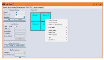
Once connected, G44H will load the settings used from last time. The default setting for the new unit out of package is 2x2 video wall with input 1 across the 4 screens. All outputs are set at resolution of 1920 x 1080@60.
