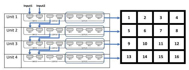
Connect all the inputs with video sources and outputs with video wall screens using professional AV HDMI cables.
