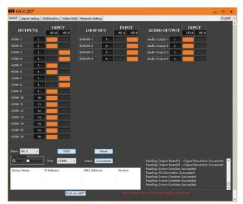
Run the G24 software and connect through RS232-control on device 1 and software will detect all 4 G24 and display 16 outputs in the software like below.
