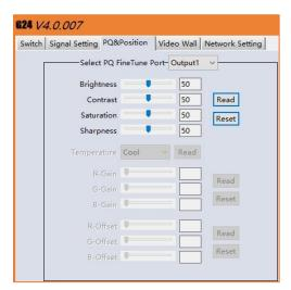
This section allows the user to fine-tune the settings of their screen from the G24H software.
