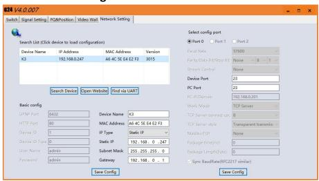
Users can find all the device network information in this section and do the modification if needed.
