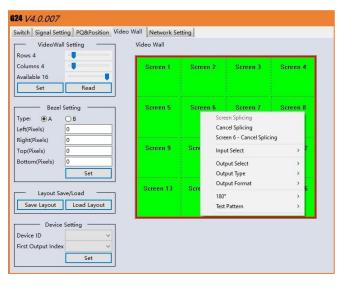
In Video Wall, set up the desired video wall layout by choosing the correct Rows and Columns in Video Wall Setting.
