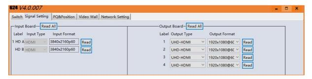
**Signal Settings** tab, users can use the **'Read All'** function button to recognize the type and resolution automatically. Additionally, you can also manually read one Input/output at a time – pressing the **Read** button next to the selected input will only read that input alone.
