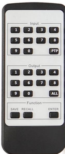
Press OUTPUT a + INPUT b + Enter to switch input b to output a
