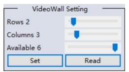
Users can set up the layout of the video wall in 'VideoWall Setting' by simply choosing how rows and columns in the video wall. Total screens amount is up to 8 for G88 video wall controllers.
