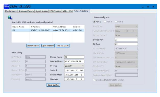
Users can find all the device network information in this section and do the modification if needed. Users can find the lost IP address using 'Find via UART' which only requires RS232 connection.
