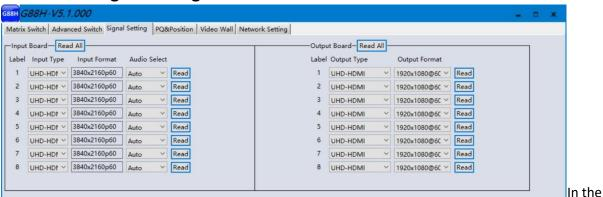
**Signal Settings** tab, users can use the **'Read All'** function button to recognize the type and resolution automatically. Additionally, you can also manually read one Input/output at a time – pressing the **Read** button next to the selected input will only read that input alone.
