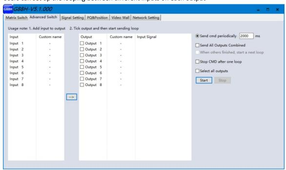
The **Advanced Switch** tab will repeatedly send a batch of command lines at the interval time specified in 'Send cmd Periodically'
