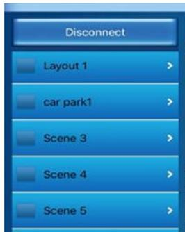
It has 40 preset buttons to recall all the preset layouts saved using SW-Control on this very SW video wall controller. Users can recall the preset layout by double tapping the very layout.
