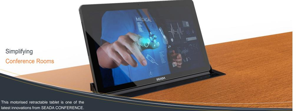
This system can be used as a standalone unit in class rooms, offices, receptions etc. It can be used not only as a tablet but also a PC. In addition it can operate as a multi units' system with the SEADA paperless conference platform. SEADA conference platform has multiple screens across the table which allows all the participants to have a clear view of the information.
