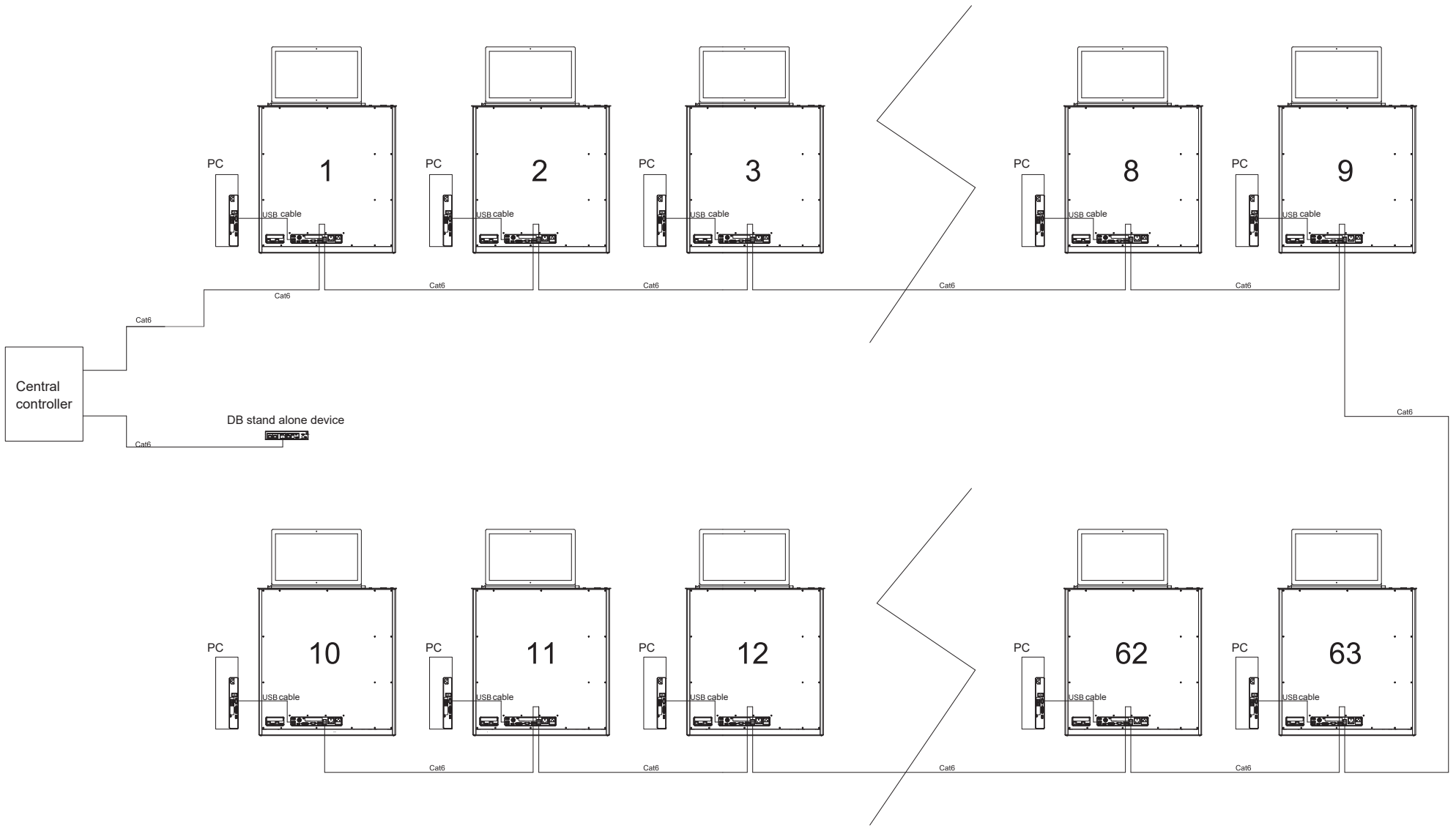
RS485 connection diagram
