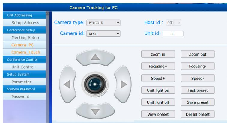
**CAMERA\_PC & CAMERA\_TOUCH** are offering the same camera setting function, but Camera\_Touch version is optimized for mobile devices user, it has touch release time (**BUTTON TIME**) adjustment option, user may choose it to operate as needed.
