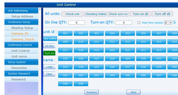
**UNIT CONTROL** interface allows operator to check the real time status of each microphone unit connected to the system. Unit ID will indicate in green color when it is in use, clicking the unit ID can control the ON & OFF of corresponding unit.
