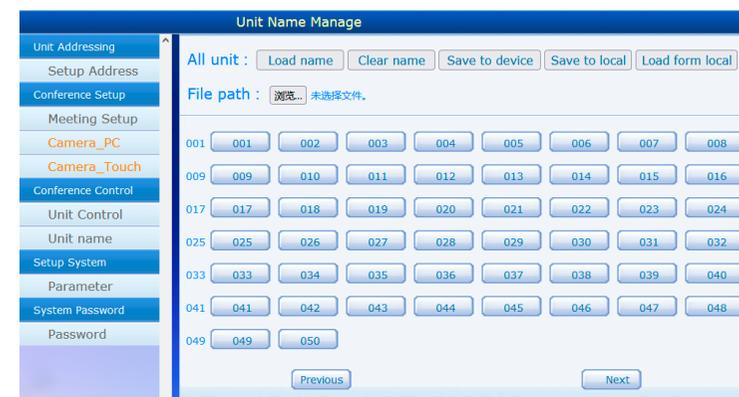
**UNIT NAME** interface allows operator to enter the name of attendee by clicking the unit ID, then click “Save to device” to save as default name list. When user leaved this section and come back to this page, name list will not display until clicking “Load name” to retrieve the default list.
