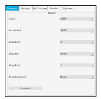
To successfully connect select correct port and make sure that all settings are as below:
