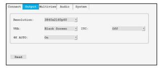
In 'Output' tab user can change the resolution, select VKA mode between Black Screen or Blue Screen, and Disable 4K Auto function.
