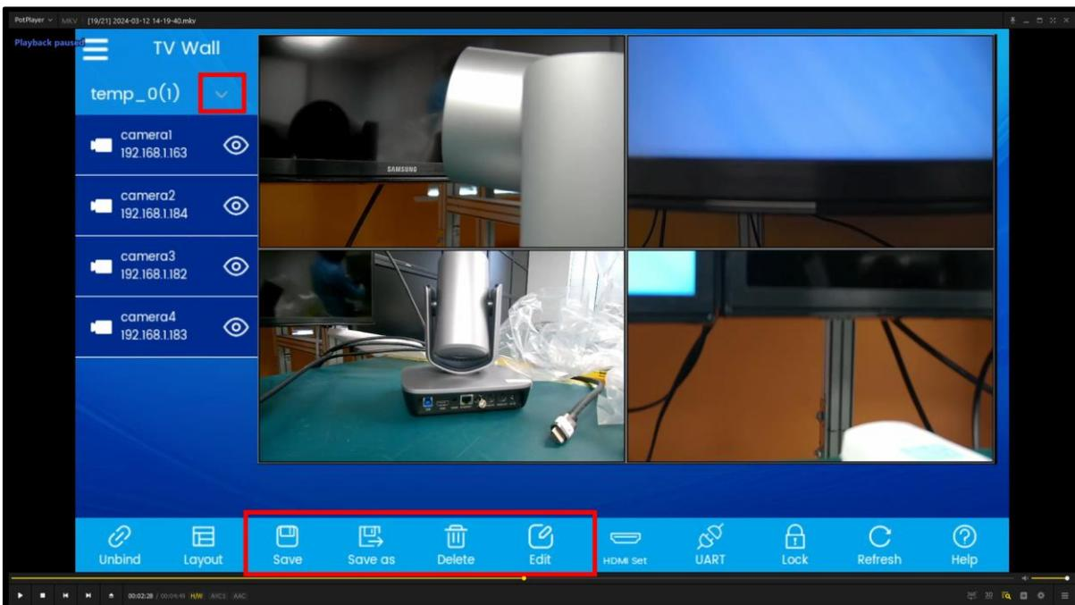
TV Wall mode is mainly used for management of a large number of cameras. In addition to basic functions in PTZ mode, TV wall mode contains the following extra functions:
