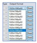
Users can manually change the output resolution here to match the requirement of the receiving side
