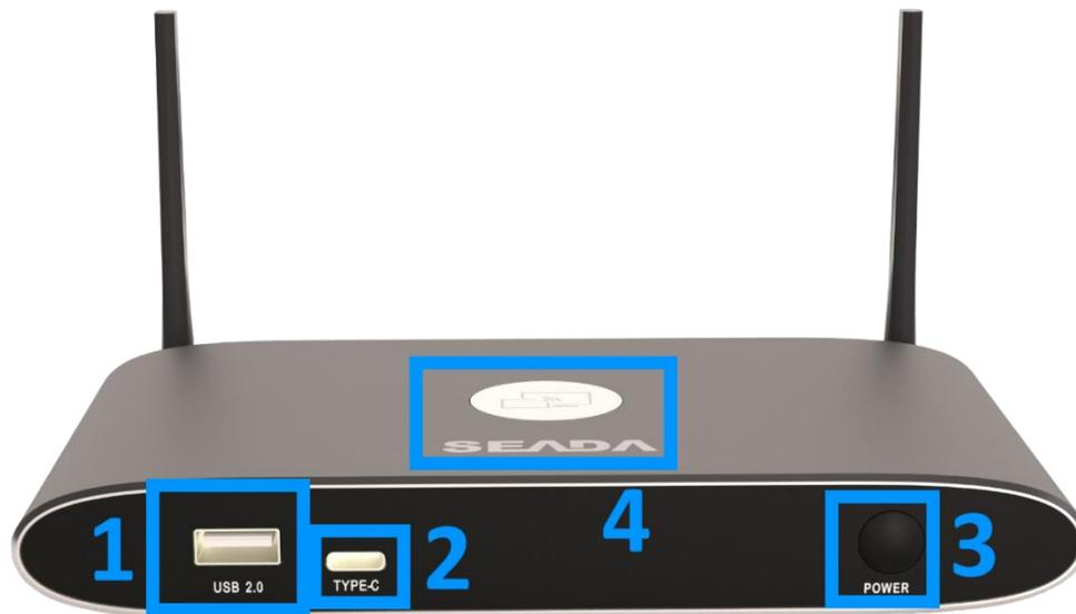
**Note:** Front USB port and type C port cannot be used at the same time, type C port is prior to USB port.
